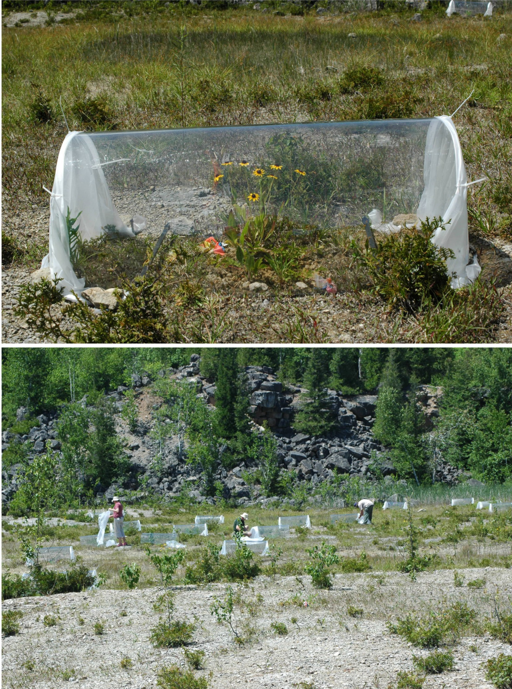
Plate 1. Photographs of quarry floor plots in the perturbation treatment receiving Climate Change Structures (CCS). Structures were installed at 50 plots randomly located across the Waters quarry site on 28 June 2007 (top panel) and removed on 2 September 2007. Each CCS, designed to block infiltration of precipitation and retain thermal radiation, consisted of a 1.2 m X 1.2 m sheet of transparent polycarbonate folded and bound into a half-cylinder shape using rubber straps and plastic cable ties, centered over experimental alvar-seeded plots, anchored using steel stakes and rocks, and covered-over at open sides with polyethylene sheeting (bottom panel).
