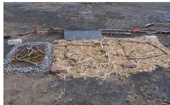
Figure 4-19. Images of the experiments on the effect of a sheltering topography. Left: experimental plot with subplots showing contour ridges and moss introduction areas with two species. Right: two subplots, one with a contour ridge and the other without, are covered with straw mulch.
