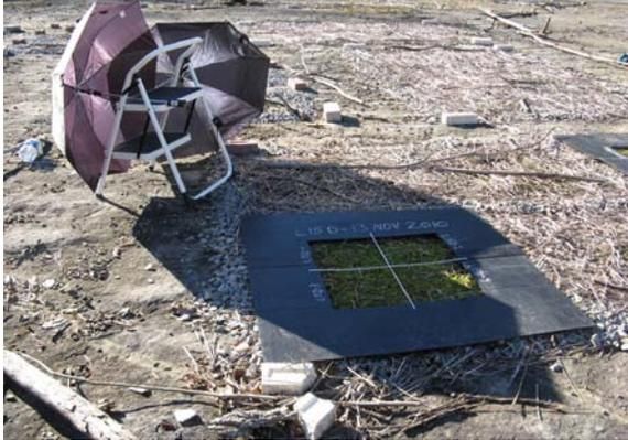
Figure 4-20. Cut-out plastic sampling frame. Umbrellas were used to evenly shade the plots when taking pictures, for better results.
