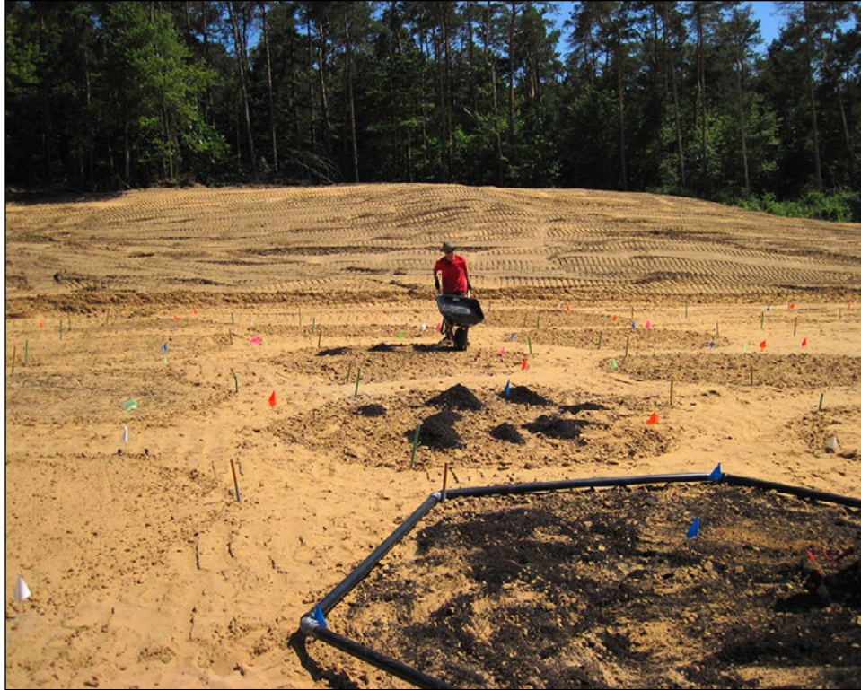
Photo: Incorporating soil amendments into pit floor substrate. Each 10^2 meter plot will have 72 tallgrass prairie plant plugs. (Photo taken May 2010)
