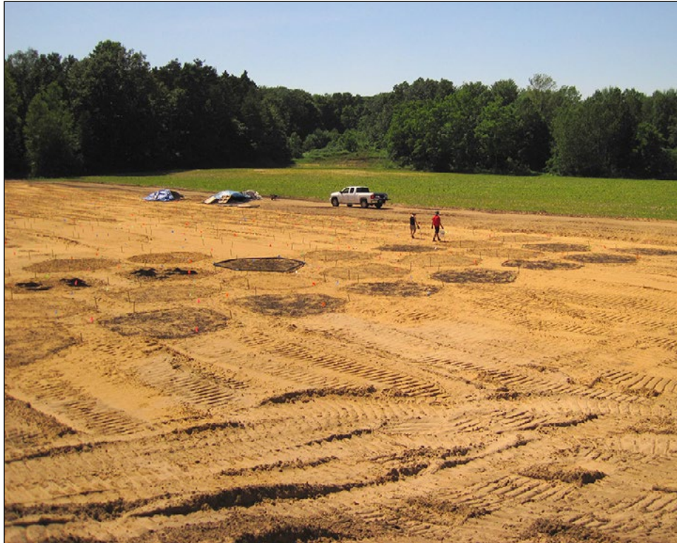
Photo: Progress of amendment application. The dark hexagon has soil amendment mixed into the upper layer of pit floor substrate. In total, 150 plots were established for the plant plug experiment and 72 plots for the seed experiment. (Photo taken May 2010)
