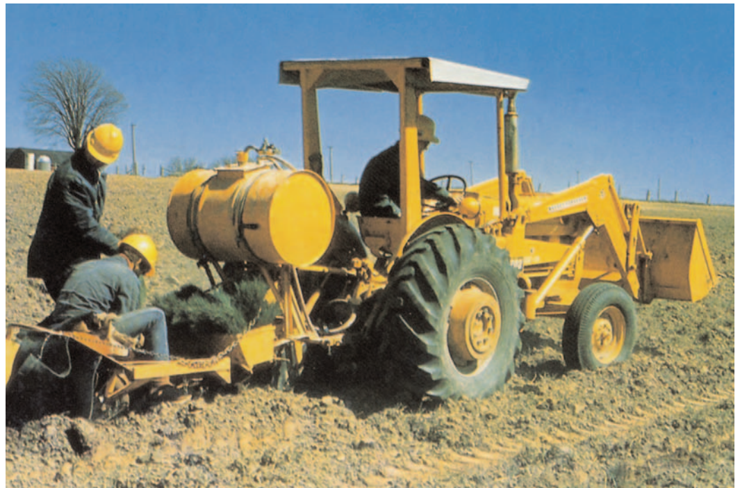
Figure 10. Machine planting is cost effective when the area to be planted is larger than 4 ha.
