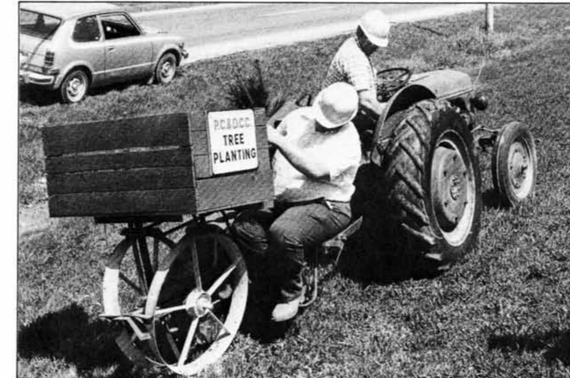
Planting bare-root seedlings of forest species with a tree-planting machine. (Port Colbourne Quarries Ltd.)
