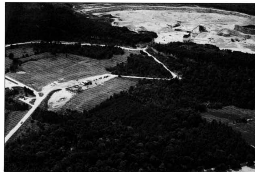
Site design to take advantage of existing vegetation: haul routes through natural woodland are visible from the air only. (Dufferin Aggregates)
