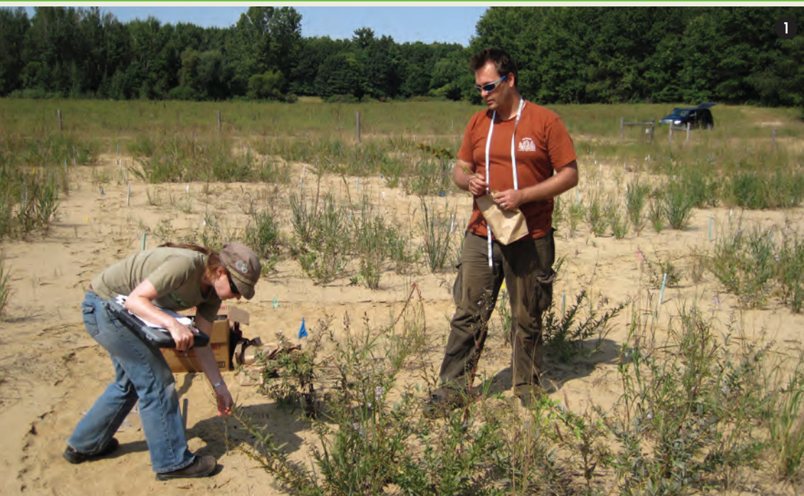
2. A variety of measurements were used to predict plant biomass. In this photo, Jeremy is displaying our weighted plate apparatus. To measure a plant, the weighted plate is dropped onto a plug of interest. The height of the plate is recorded. Weighted plate measurements strongly correlated with dry plant biomass for the C3 and C4 grasses.
