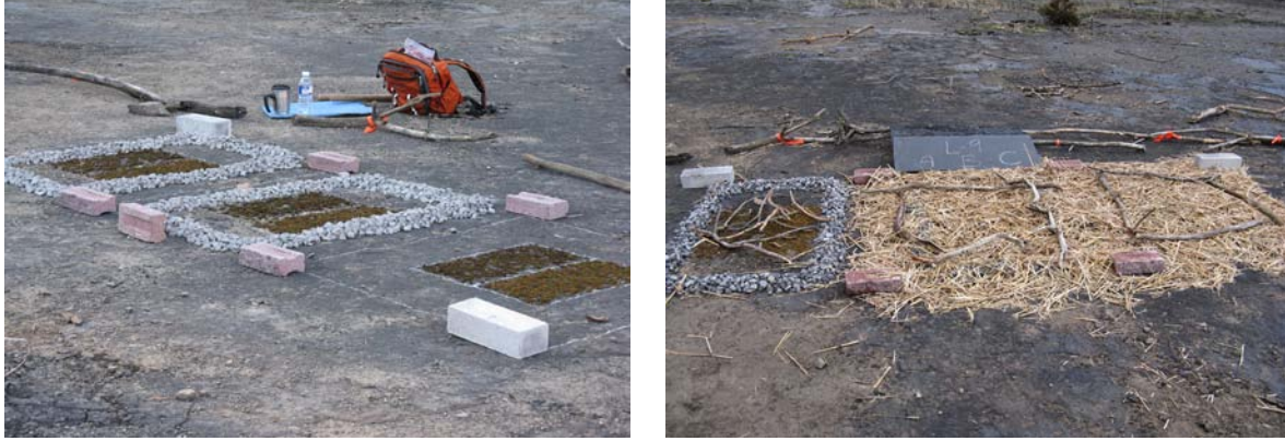
Figure 18. Images of the experiments on the effect of a sheltering topography. Left: experimental plot with subplots showing contour ridges and moss introduction areas with two species. Right: two subplots, one with a contour ridge and the other without, are covered with straw mulch.
